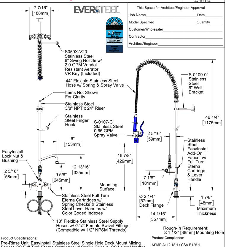
Faucet, SS Full Turn Eterna Cartridges w/ Spring Checks, SS Lever Handles,
